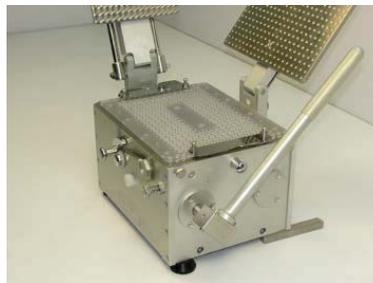
**2.** Place the OE Guide Tray onto the Filler. Steps for caplet orientation are similar to capsule orientation.
