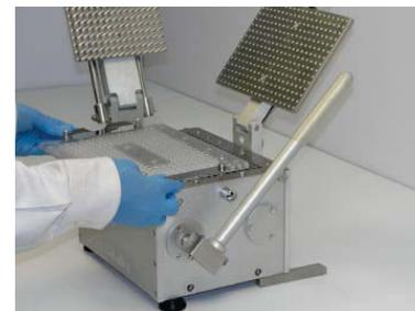
9. Remove the Caplet Orienter Base, Caplet Tray and OE Guide Tray. Continue with Operating Instructions in your ProFiller 3700/3800 Manual. Begin with "Filling Capsules" if adding an excipient (page 18 in Manual v 1.2.1), or continue with "Locking Capsules" to lock the outer capsules (page 20 in v 1.2.1).
