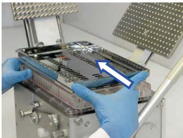
7. Push sliding portion of Caplet Tray to the left to drop the caplets into the capsules.
