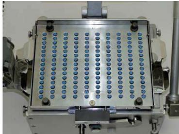
7. For sizes A, B and D only, remove ATF and repeat steps 3-6 except in step 5 place the ATF locating studs into the second holes of OE Guide Tray. Repeat steps 3-6 a third time, placing ATF studs into third holes in step 5.
