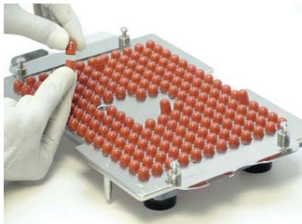
**7.** Capsules that have not separated will be pushed higher up in Caps Tray. Remove these capsules and separate the cap from the body by hand. Insert the cap back in the Caps Tray and insert the body into the Filler.
