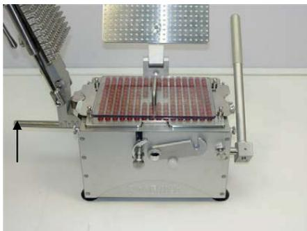
1. Make sure Cam Handle is at 0° on cam indicator. Place loaded Caps Tray with Push Plate onto Filler.
