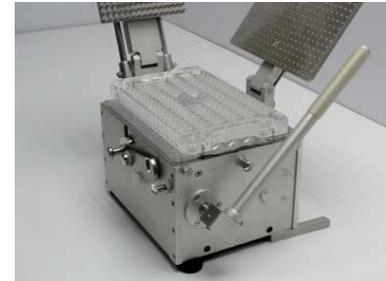
3. Place the Capsule Orienter Base on the OE Guide Tray. Align the front edge of the Orienter Base with horizontal line I on OE Guide Tray. Align the right edge of the Orienter Base with the right edge of the OE Guide Tray.
