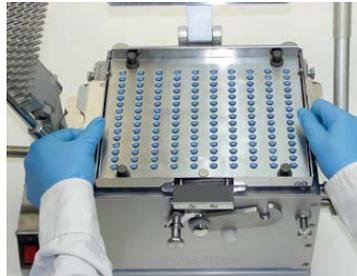
5. Place ATF locating studs into front holes of OE Guide Tray.
