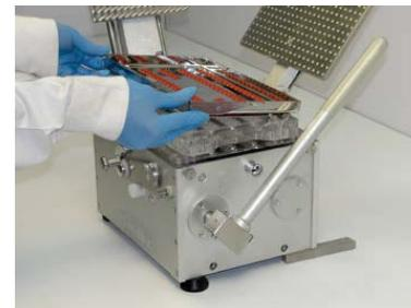
6. Place Caplet Tray on Caplet Orienter Base and slide back until it drops into place.
